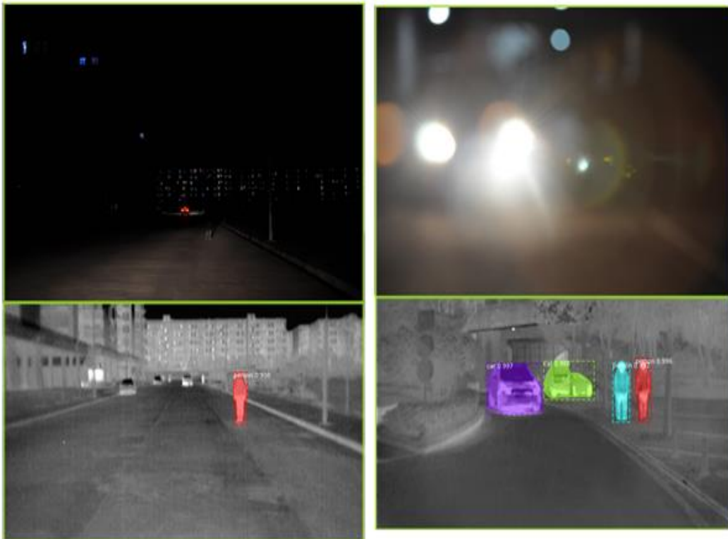
Figure 5-2. The top part of the image is RGB, while the bottom is an IR image of the same position and time.
