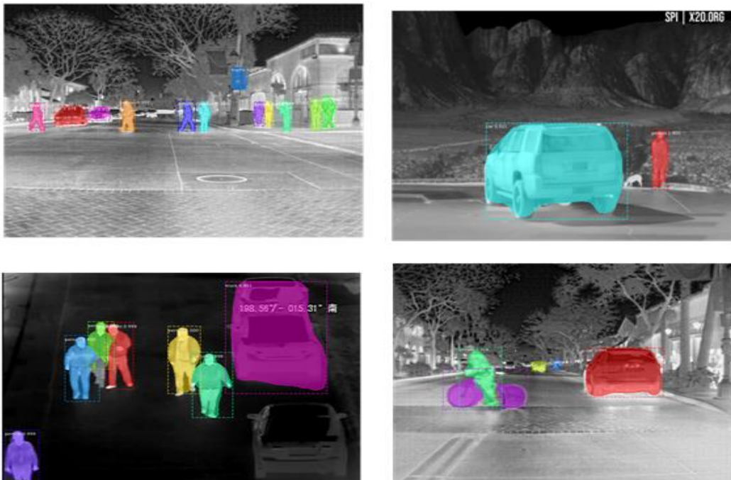
Figure 5-1. Detection and instance segmentation of dim target objects in infrared using Mask R-CNN
