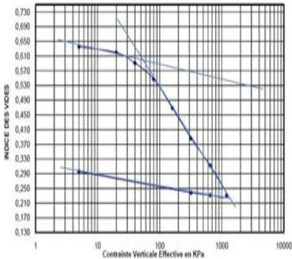
Figure 3. Compressibility curve by oedometer test conducted in the laboratory
