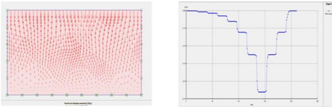
Figure 5. Simulation inputs: on the right, curve of displacements in function of steps, on the left the vertical displacement of the soil sample.
