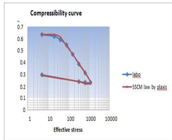
Figure 7. Compressibility curves by SSCM law (plaxis) and laboratory test
