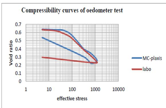
Figure 6. Compressibility curves by mohr coulomb law (plaxis) and laboratory test
