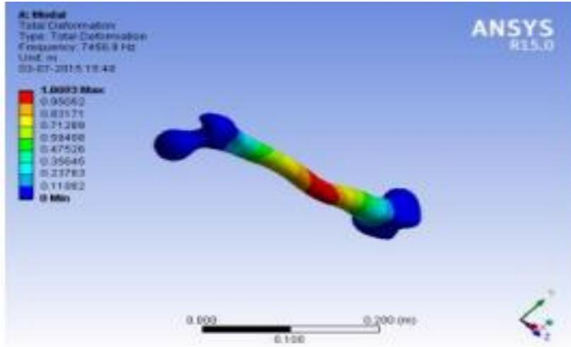
Figure 2. Mode Structure 1 for fixed-fixed boundary situation
