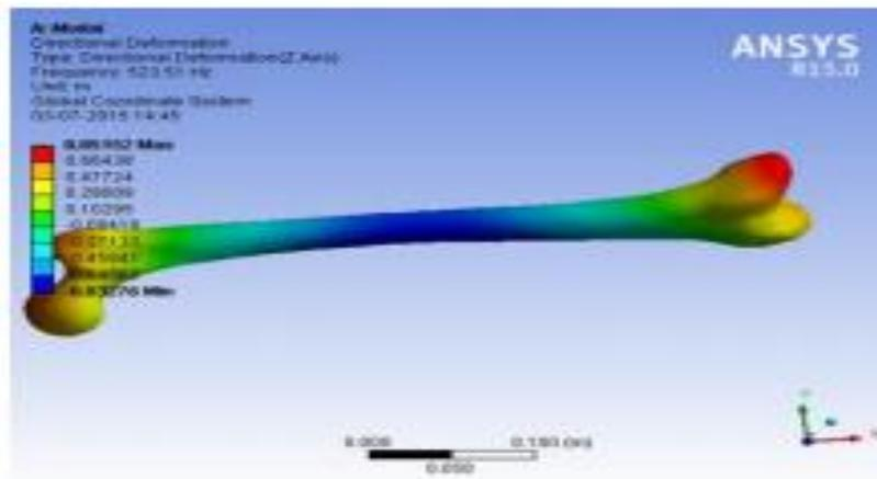
Figure 3. Mode Structure 8 for free- free boundary situation
