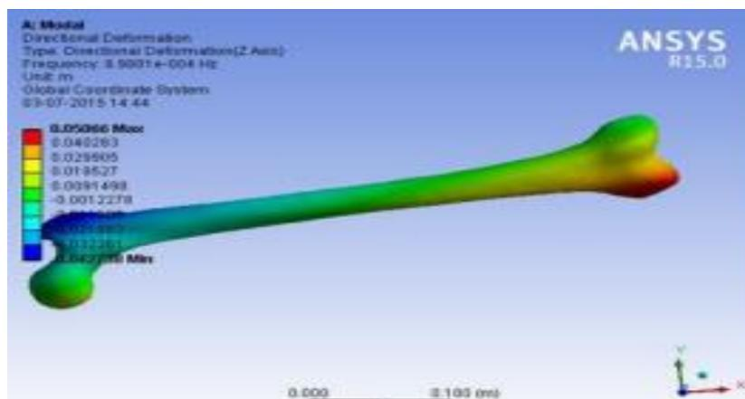
Figure 1. Mode Structure 6 for free-free boundary situation
