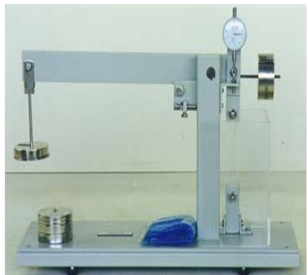
Figure 2. Perfect Connected Structure of creep testing machine
