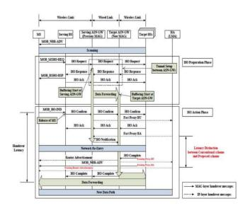
Figure 5. Layer3 handover for mobile WiMAX based WMN [4]
