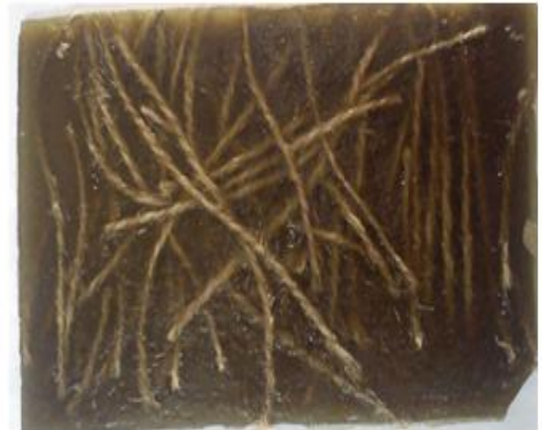
Figure 2. Composite with Jute fiber and Synthetic Resin
