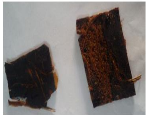
Figure 3. Composite with jute, banana fiber and blended resin
