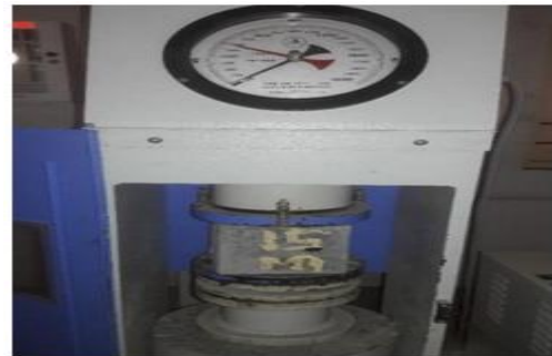
Figure 2. Compression test Setup
