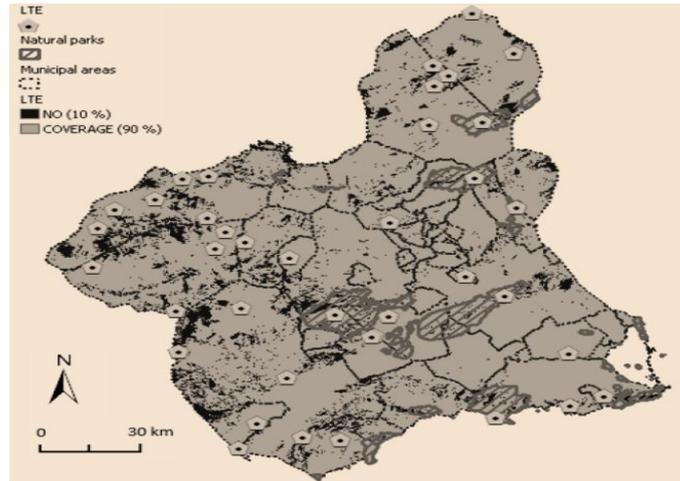
Figure 7. LTE optimized radioelectric coverage (39 sites)
