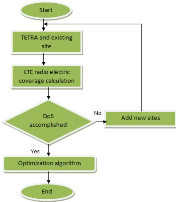
Figure 5. The proposed flow-chart to plan the new LTE network.
