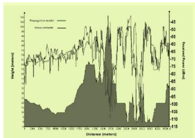
Figure 4. Comparison between measurements and propagations model
