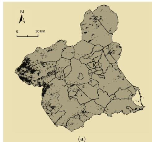
Figure 6. Radioelectric coverage for (a) the TETRA system (16 sites)
