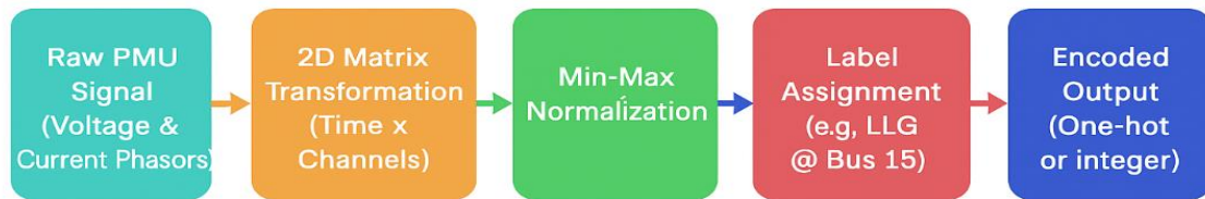
Figure 3. Data preprocessing pipeline from raw PMU signals to deep learning-compatible input matrices for fault detection
