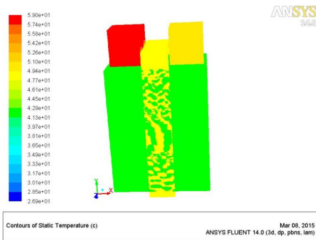
Figure 5. Temperature distribution using conventional material LiCoO4 under steady state condition after 5p discharge rate
