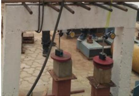
Figure 2. Experimental Setup of Monolithic Frame
