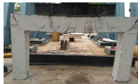
Figure 5. Represent Crack Pattern in Beam of Specimen
