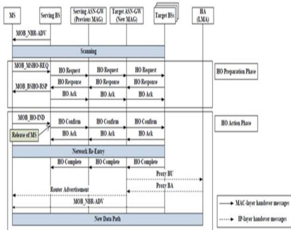
Figure 4. Layer 3 Hand over procedure [4]
